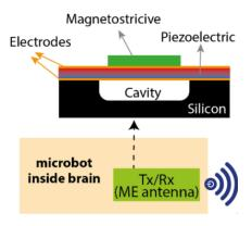
Figure 1: Schematic of cross-section of the magnetoelectric (ME) antenna
